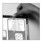
•Mount the metal stays to the slots, inside of the cover, after taking them out from the plastic holders. Push the lock to close.
